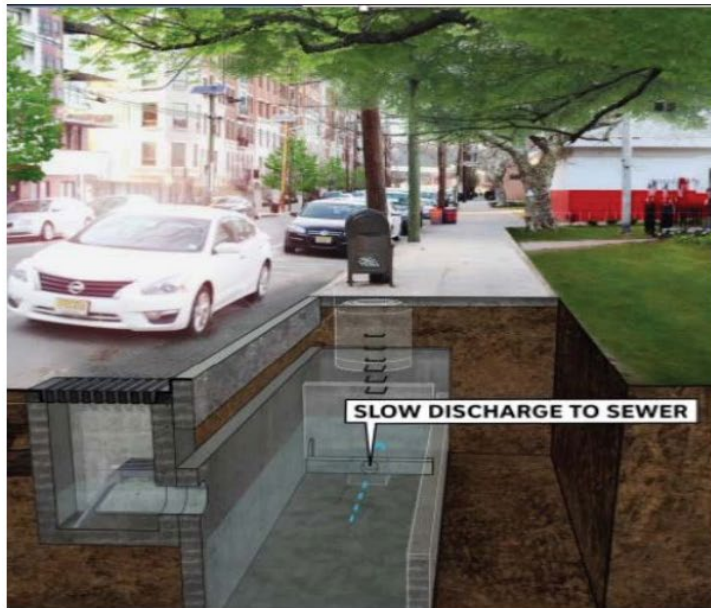
Figure 4-20: Schematic for typical stormwater retention system depicting tanks and typical “High Level” storm sewer system for three DSD sites.
